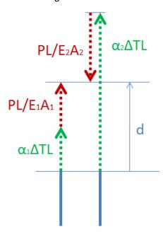
These equations are valid throughout the elastic range of the materials. When the increment of temperature is enough the P load will get a value that will pass the yielding stress of the material of one bar (bar 1 for example):
